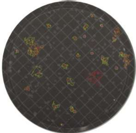
Figure 6. Top pictures show images of the black gridded membranes taken by the ScanStation®. Bottom pictures show the images after being processed by the software for enumeration of CFU (visualization of crosses and detection area around colonies). The camera configuration is black background.
